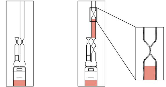
Seal Configuration for No Segment    Seal Configuration for Segment    Seal Close-Up View
